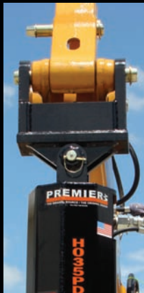
Pin-On Mounts - available for any excavator. Contact factory with make and model for specific part number and pricing.
